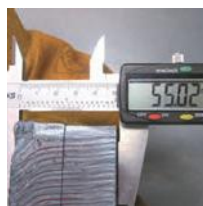
Carbon Steel Max. Cutting Thickness: 55 mm
