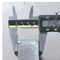
Carbon Steel Max. Cutting Thickness: 35 mm
